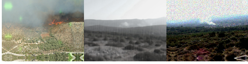
Fig. 6: Some examples for data augmentation over the wildfire dataset. From left to right: Random color blurred glares and affine translation with edge mirroring; gaussian blur, rain and desaturation; random noise and affine translation with edge mirroring.
